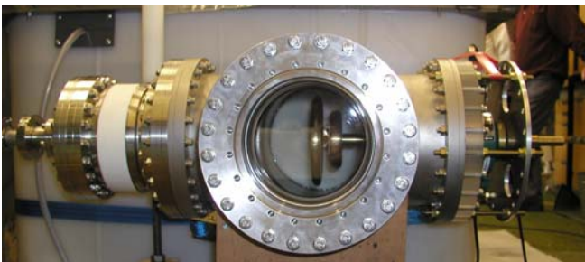
Fig. 8 (left) Vircator HPM generator; (right) overall view of complete system
