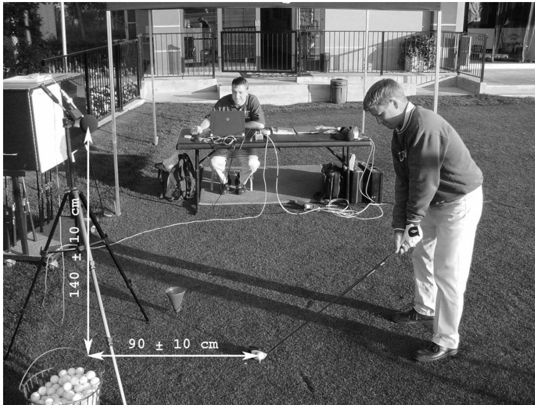
Figure 1. Microphone location in the test set-up
