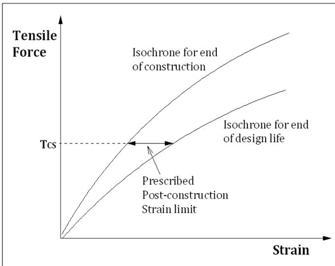
Figure 4. Typical isochronous curve used for restricted service tensile stress capacity. Adapted from BS 8006 (2010).
