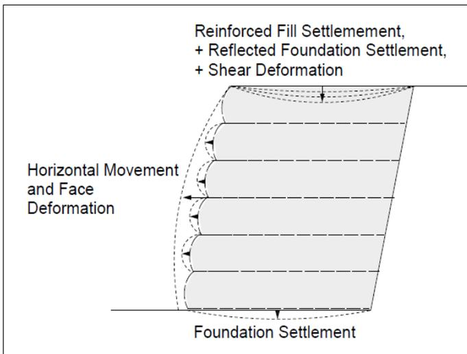
Figure 2. Sources of post-construction deformation in a typical GRSRS according to EBGEO (2011).
