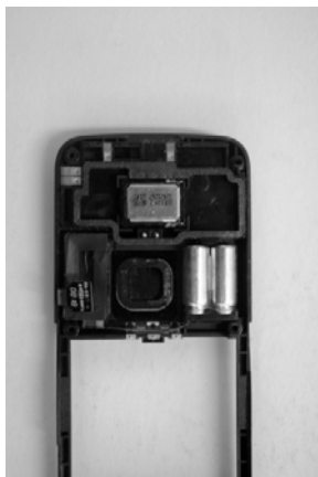
Figure 2. Antenna location of the Nokia 6220c
