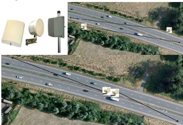
Fig.8. Directional antenna and their locations
