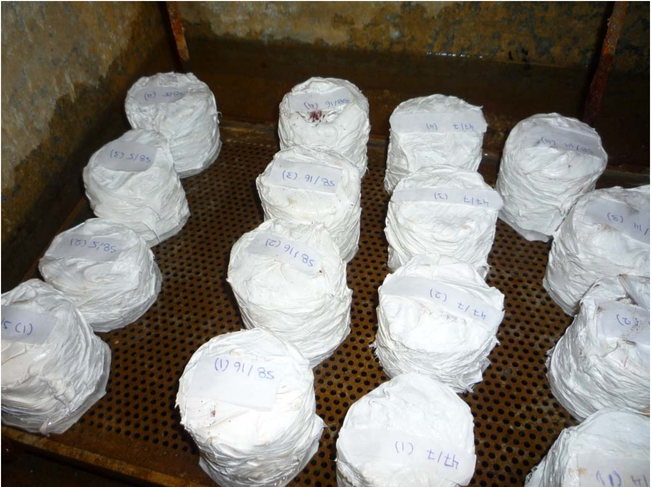
Figure 6: Cores sealed with proprietary polysulphide sealant for capillary absorption testing
