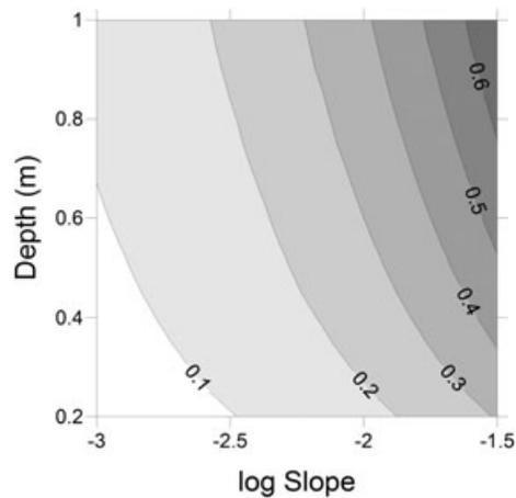
**Figure 6.** Absolute differences in velocity ( $\text{ms}^{-1}$ ) estimated using a Keulegan-type approach for surfaces of different  $D_{84}$ . Differences are estimated for ranges of slope and depth values that are reasonable for gravel-bed rivers using, as an example, the difference in  $D_{84}$  between casts 3 and cast 4.
