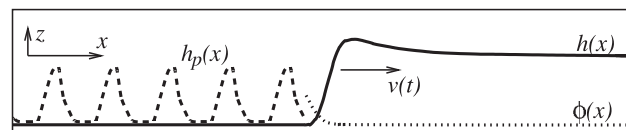
FIG. 1. Sketch of a liquid front that recedes due to evaporation and convection with a varying velocity v(t) . The deposition process is characterized by the film thickness profile h(x, t) , the concentration profile \phi(x, t) (in the bulk film), and the particle layer thickness h_p(x, t) = \phi(x, t)h(x, t) (outside the bulk film).
