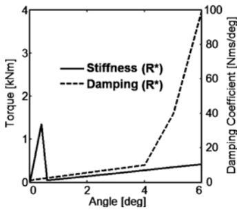
Figure 8 Stiffness and damping functions for R\*.
