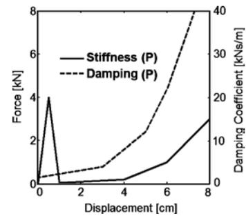
Figure 9 Stiffness and damping functions for P.
