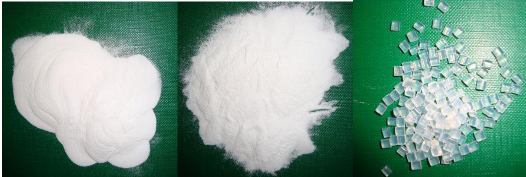
Figure 1 PA 12 samples used in the study: (a) PA 12 used powder; (b) PA 12 virgin powder; (c) PA 12 granules for injection moulding
