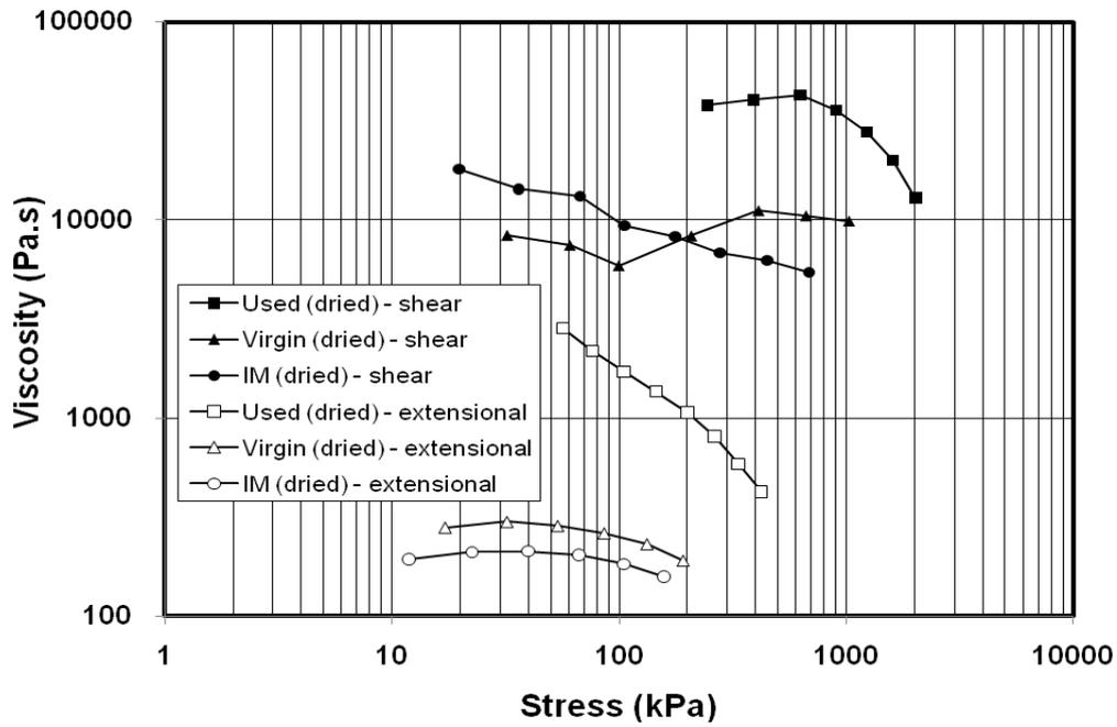
Figure 9 Composite plot of viscosity data for PA-12 polymers at 200 °C: shear and extensional flow data from capillary rheometry.
