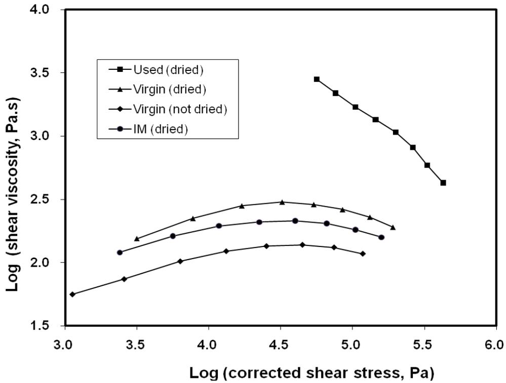
Figure 5 Shear viscosity data from capillary rheometry at 200 °C for PA-12 polymers, plotted as shear viscosity versus shear stress.
