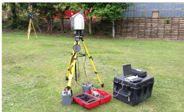
Figure 3. Typical Laser Scanning Equipment with HDS target in the background
