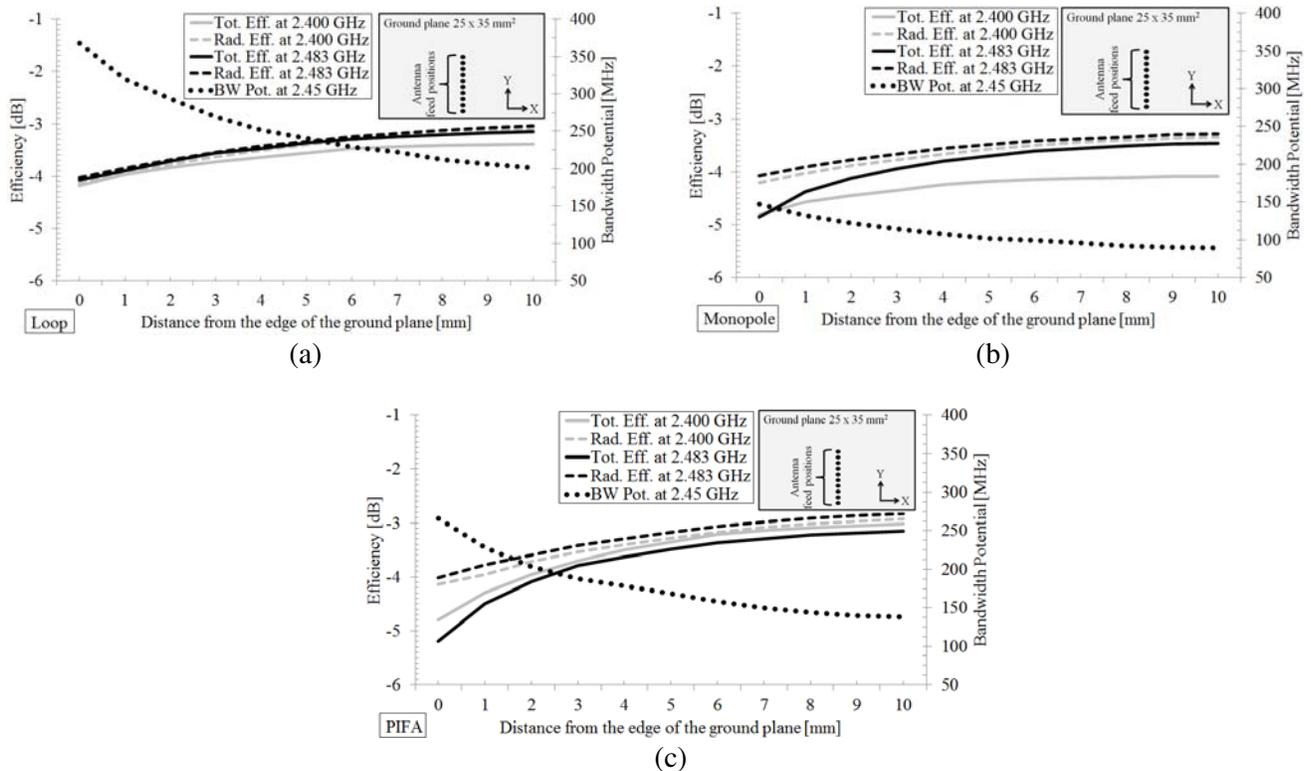
**Figure 4.** Total antenna and radiation efficiencies [dB] presented together with BW potential [MHz] as a function of the antenna feed point distance from the edge of the ground plane for (a) loop, (b) monopole, and (c) PIFA.
