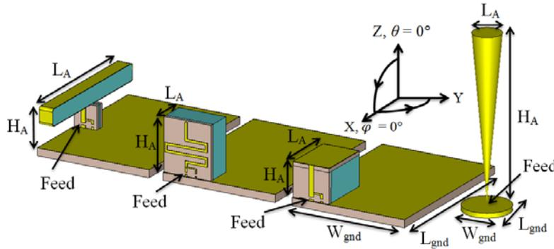
**Figure 1.** Oblique views to show feeding positions and to indicate the size of the antennas to cover the spectrum at 2400–2483 MHz: on-ground loop, monopole and PIFA, and reference disccone. A blue support material is modelled by  $\epsilon_r \approx 1$  and  $\tan \delta < 0.002$  below 11 GHz, the dielectric below of a ground is made of FR4 (grey) and the conductive parts are of copper (yellow).
