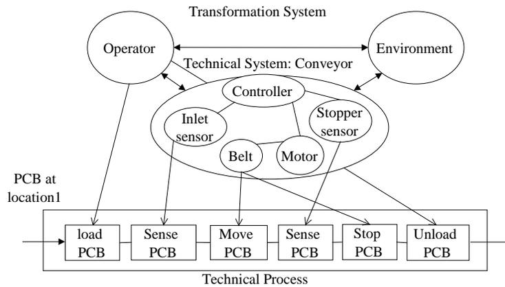
Figure 2. Transformation Model for Conveyor
