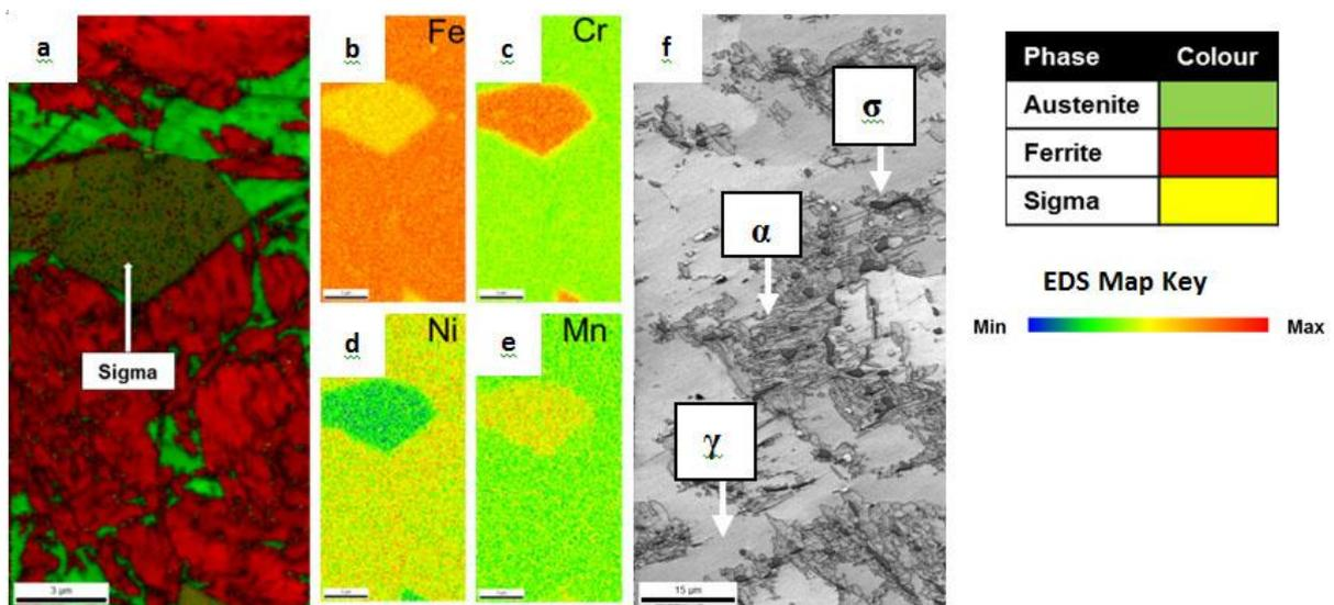
Figure 8: (a) EBSD phase map of a  $\sigma$  particle that has formed on the austenite/ferrite interface in the 321 parent metal after ageing for 12000 hours at 750°C with accompanying EDS maps (b-e). (f) EBSD image quality map of the weld metal after ageing for 12000 hours at 750°C,  $\sigma$  has formed on the austenite/ferrite boundaries and also in the prior delta ferrite regions.
