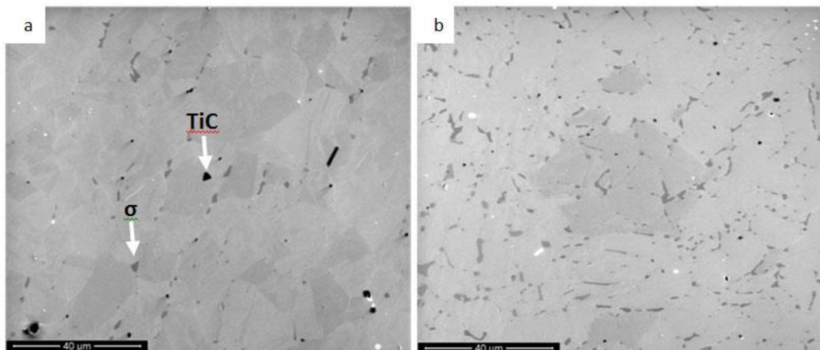
Figure 5: Ion beam images of the parent (a) and the weld metal (b) after ageing at 750°C for 100 hours. There are two particles, the darkest being titanium carbo-nitrides and the other is  $\sigma$ . Ion beam imaging was selected for the imaging technique for these materials as it can produce contrast between the matrix material and the second phases without requiring an etching technique which can introduce depth effects into micrographs.
