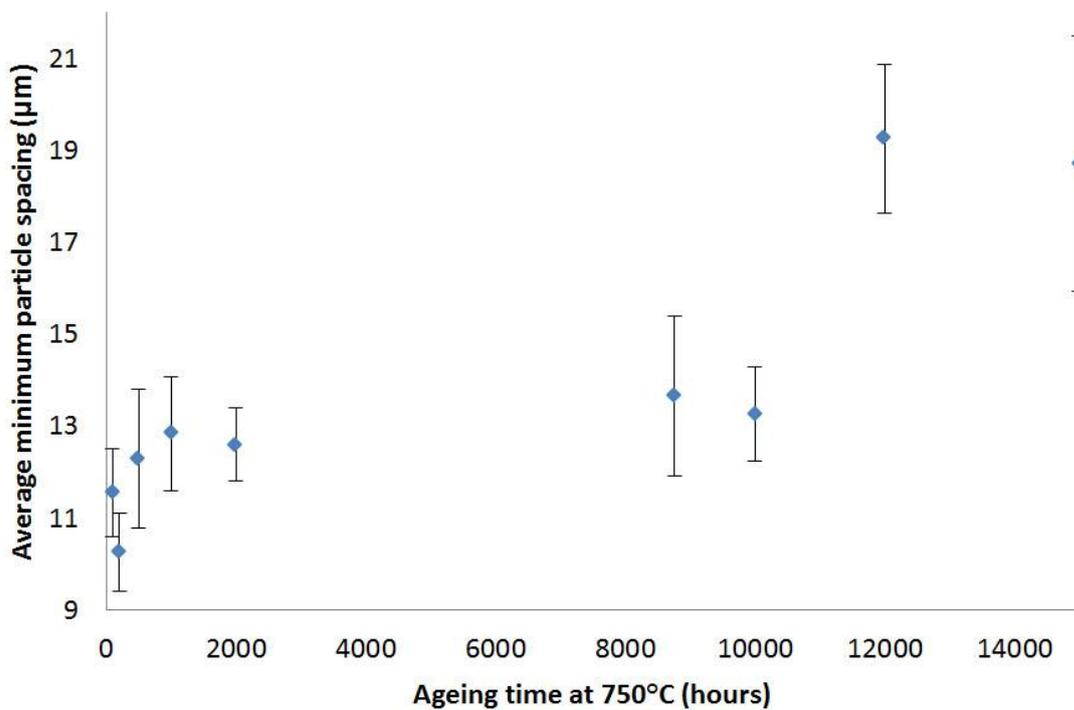
Figure 10: The average minimum particle spacing for the 321 grade parent metal determined by particle analysis of the ion beam images
