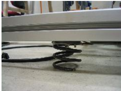
Fig. 3. Springs installed at the bottom of the platform allow small magnitude of tilting during cycling.
