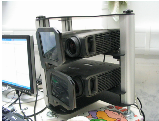
Fig. 6. Two projectors are used to produce the stereoscopic effect.
