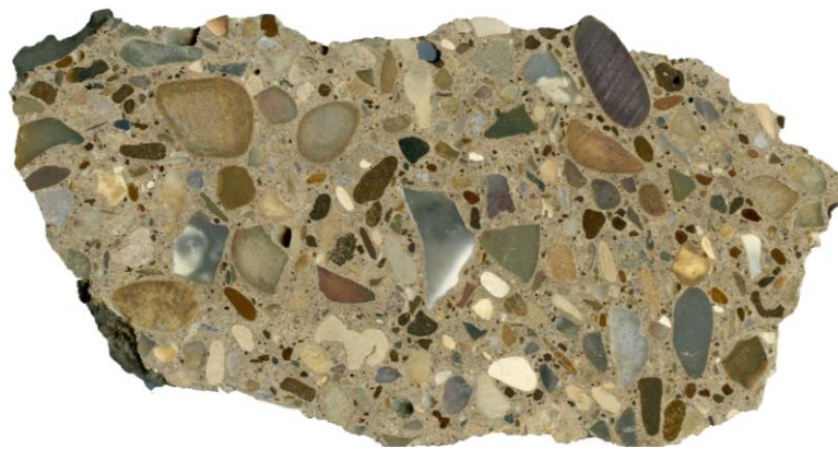
Fig. 1 - Thin section of demolition concrete for petrographic analysis [42]
