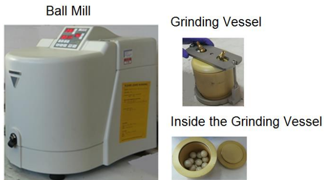
Figure 2. Ball Mill device and Grinding Vessel
