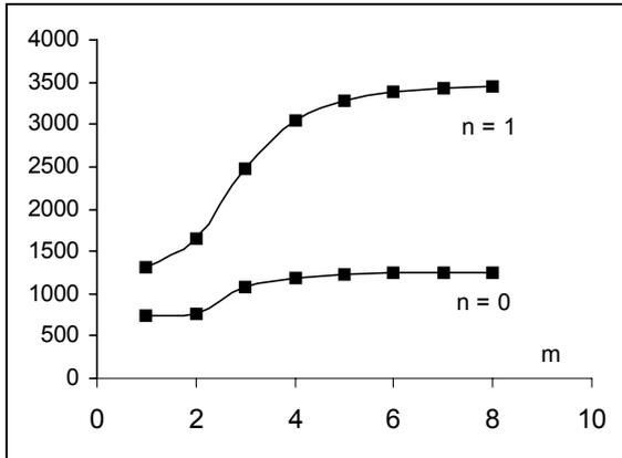
Figure 4. Frequency (Hz) v m for LUSAS predictions.
