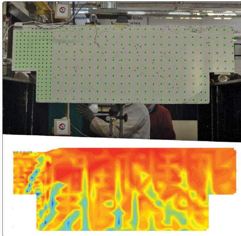
**Above: Experimental set-up and camera targets for one of the full-scale rubberised lintels tested within the structures and materials laboratory (top). Results of the digital image analysis and processing, showing presence of cracks in blue and concentration of compressive stress in red (bottom).**
