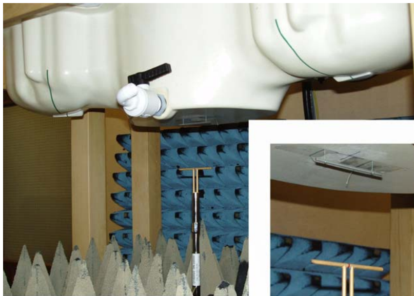
Figure 7. The measurement set-up with the DASY4 system. The 72.5mm dipole was positioned 98mm away from the flat section of the twin SAM phantom. A 70mm pin was hung 10mm below the phantom.
