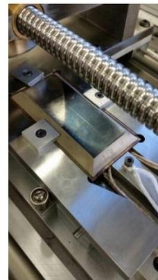
Figure 1 Slider rig used in the tests
