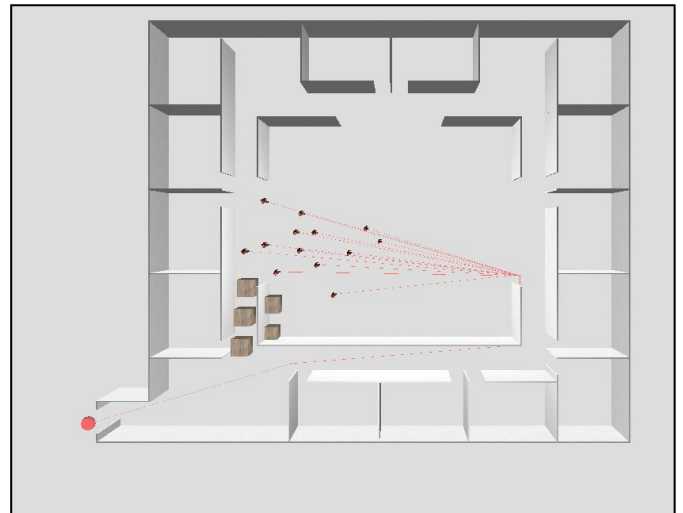
Figure 11. The shortest path blocked by boxes, AI entities finds another path to the destination point.
