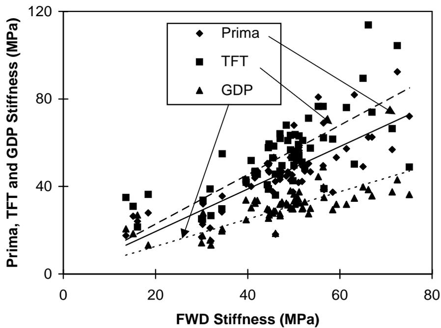
Figure 6. Relationship between Stiffness Modulus determined by the Portable Dynamic Plate Test Devices and the FWD (on subgrade and 400mm thick Granular Capping)
