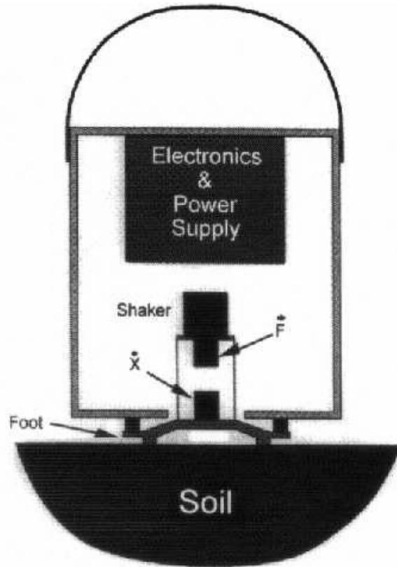
Figure 3. Schematic of the Humboldt Soil Stiffness Gauge.
