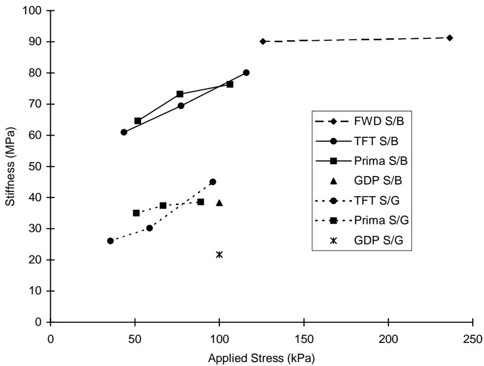
Figure 8. Relationship between Stiffness and Applied Stress for the FWD, TFT, Prima 100 and GDP on Sub-Base (S/B) and Subgrade (S/G) at a Controlled Trial Construction Site (400mm Capping and 150mm Sub-Base over a Clay Subgrade)
