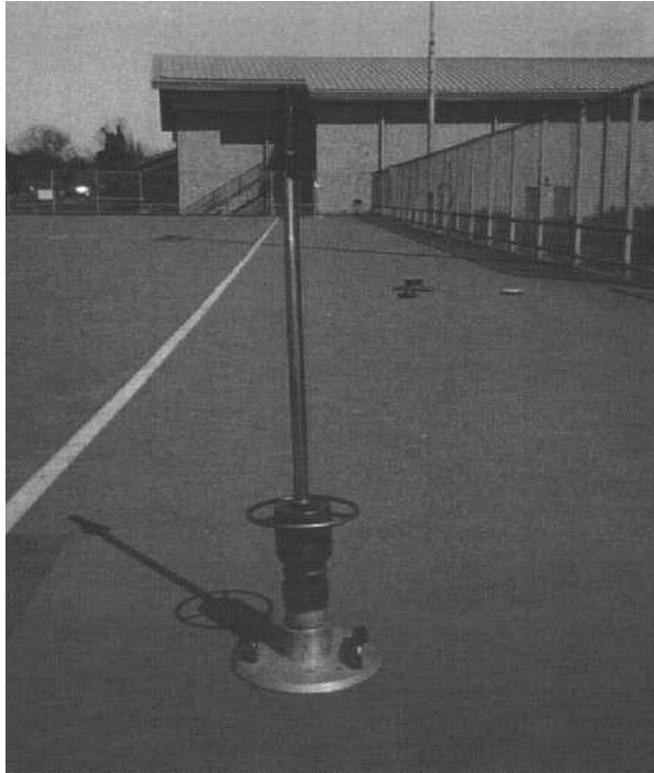
Figure 1. German Dynamic Plate test Apparatus
