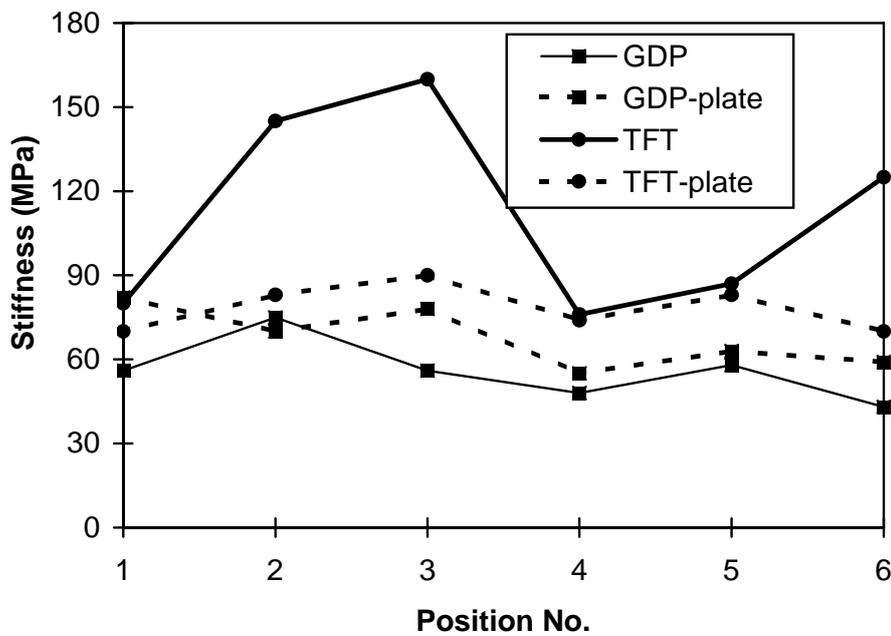
FIGURE 4 Effect of a 2<sup>nd</sup> Bearing Plate on Composite Stiffness Measurements for 550mm thick granular sub-base (Note: '-plate' = with 2<sup>nd</sup> bearing plate).
