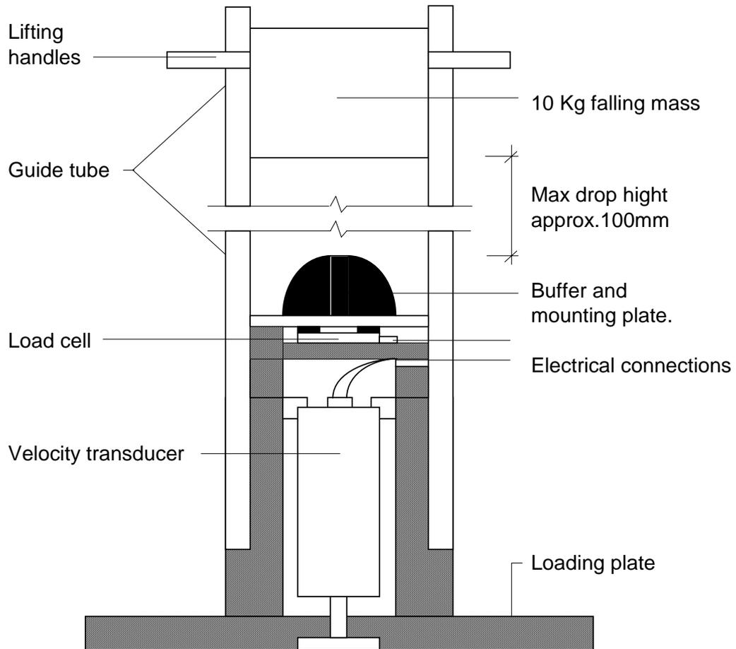
Figure 2. Schematic of the TRL Foundation Tester (TFT)
