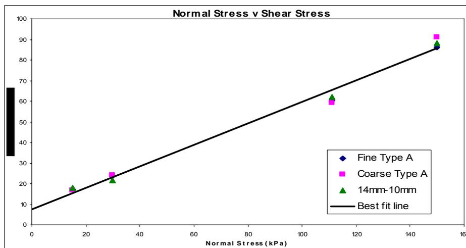
Figure 6 – Normal stress – shear stress results
