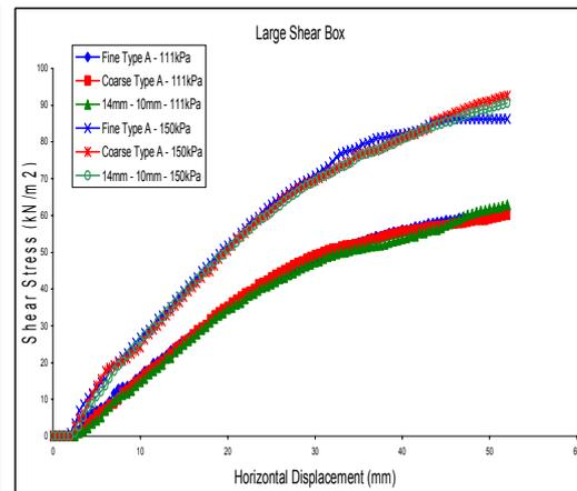
Figure 5–Stress - displacement graph (normal stress = 110kPa and 150kPa)
