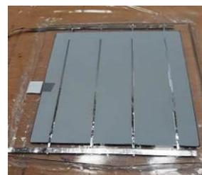
**Figure 2:** The structure of the half-encapsulated PV cells used for the investigation of the Al back contact corrosion.
