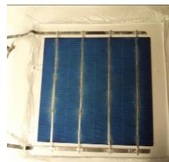
**Figure 1:** The structure of the half-encapsulated PV cells that are used for the investigation of the front contact corrosion.
