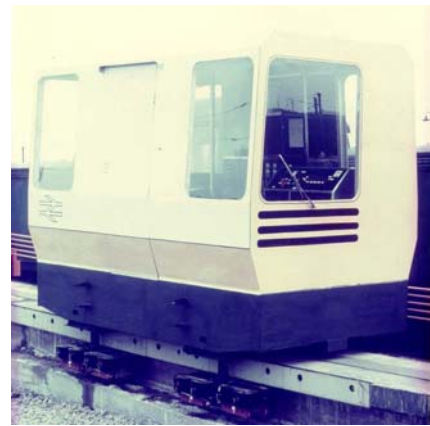
Figure 4. Low-speed 3.2 tonne Maglev vehicle
