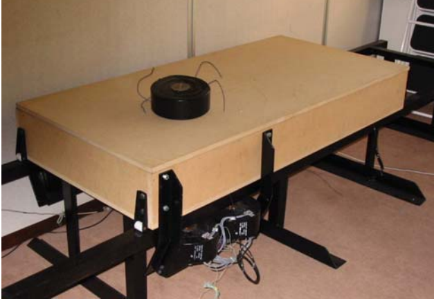
Figure 5. 200kg Maglev demonstrator vehicle
