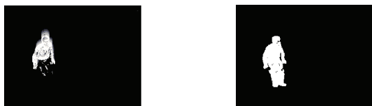
Fig. 3. MHI and background subtraction result for the sitting down case, C_{motion} = 46.20\%
