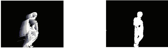
Fig. 1. MHI and background subtraction result for the fast walking case, C_{motion} = 63.55\%
