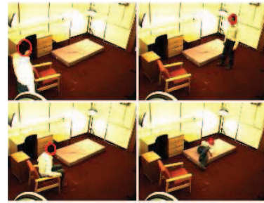
Fig. 2: Some head tracking results, the current tracked head position is highlighted by a red ellipse
