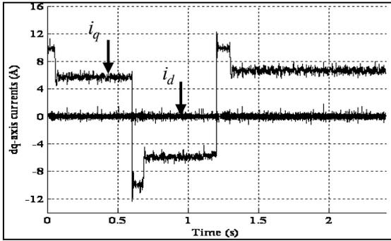
Fig. 7.  $dq$ -axis components of the armature current
