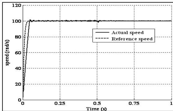
Fig. 12. Rotor speed response under load torque variation
