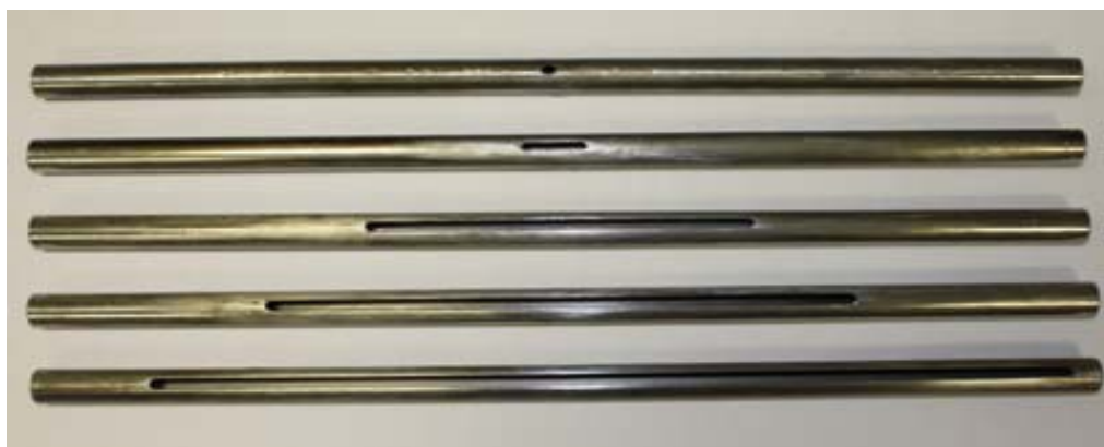
Figure 1. Photograph of steel tubes with increasing slot length; increasing from 4mm – 280mm.
