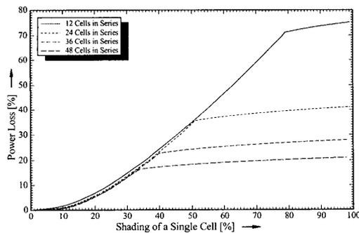
Figure 4: Power Loss Due to Shading of a Single Cell in a Module
