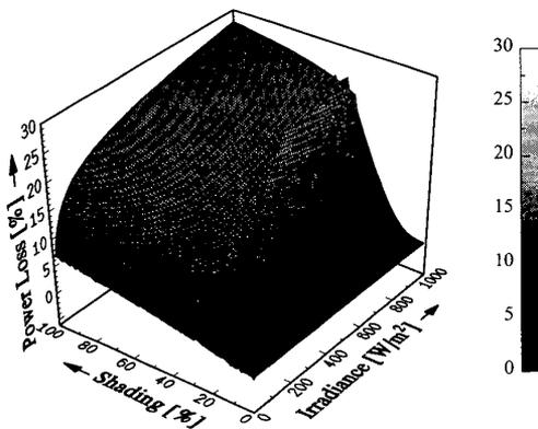
Figure 5: Influence of Irradiance and Shading on the Power Loss.
