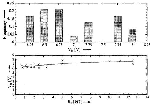
Figure 2: Histogram of Breakdown Voltages (upper plot) and dependence of the breakdown voltage on the parallel resistance.
