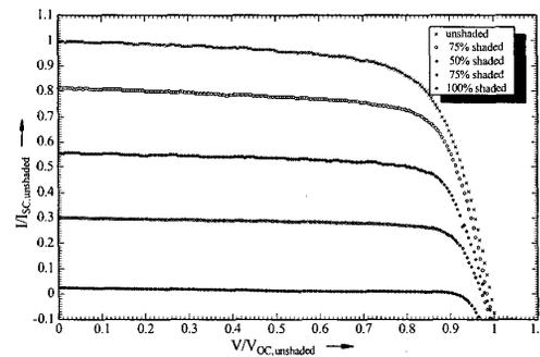
Figure 3: Measurement of the effect of shading a single cell in the mini-module.
