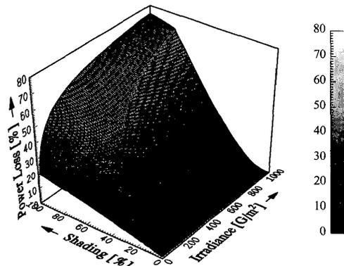
Figure 6: Power Loss of 36 Modules Connected in Series with 3 Cells Shaded.
