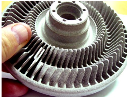
Figure 7: Laser sintered turbine manufactured in AluMide material.
