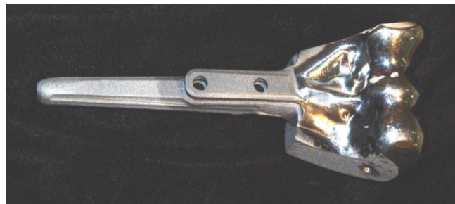
Figure 5: Titanium elbow implant manufactured after RP design verification (Truscott et al , 2007)
