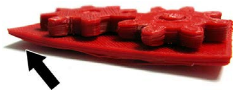
Figure 6: Warping on the base of gear system
